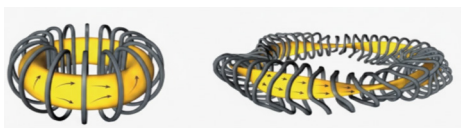
Figure 2. Comparison of magnetic confinement systems in fusion reactors: tokamak with axisymmetric toroidal coils (left) and stellarator with three-dimensional twisted coils (right) (Hambling, 2016)
